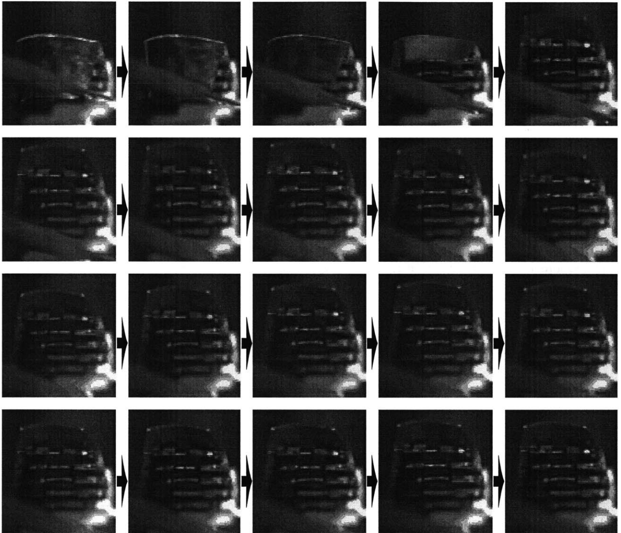
Figure 2-10: Video sequence of WASP wing response at 46 m/s and 0° root AOA with 0.006 seconds between images
