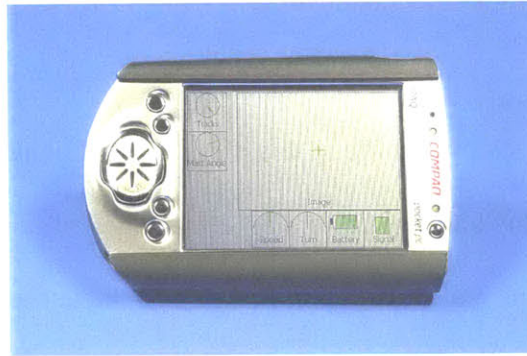
Figure 8 - Operator control interface (OCU)
