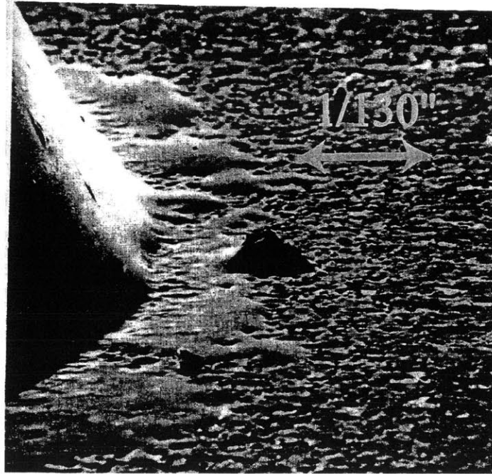
Figure 1-7: Microscopic features close to the contact line [2]. SEM picture of drop of cooled glass on Fernico metal with same coefficient of thermal expansion as glass.
