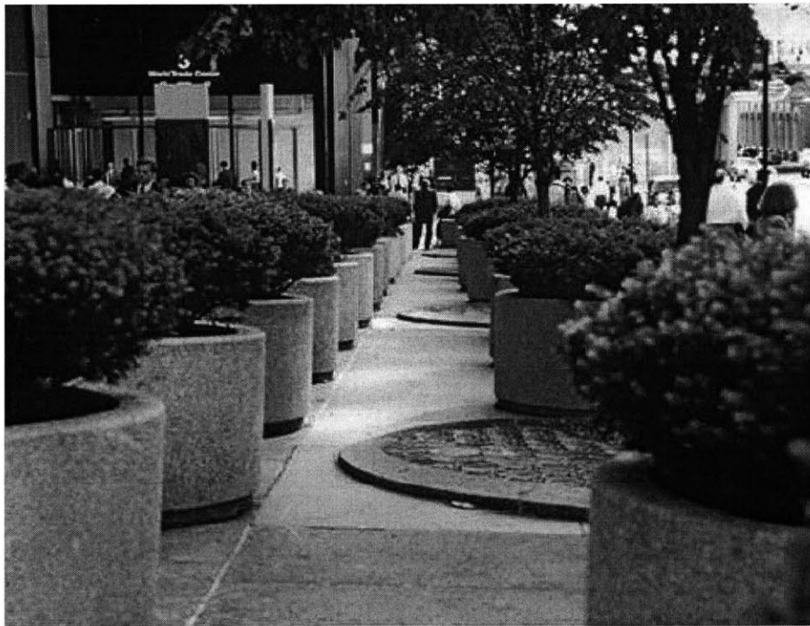
Figure 5: Planters used to increase the standoff distance.
