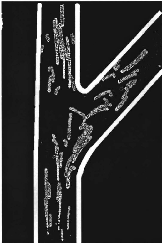
Figure 3-9: Case 11 visualization. Mother vessel: Taper , Daughter flow: 95% , Collateral flow: 0 . (A) Waveform: Dashed circle: PIV, Single circle: Streamlines at acceleration, Double circle: Streamlines at deceleration. (B) PIV. (C) Streamlines at acceleration. (D) Streamlines at deceleration.
