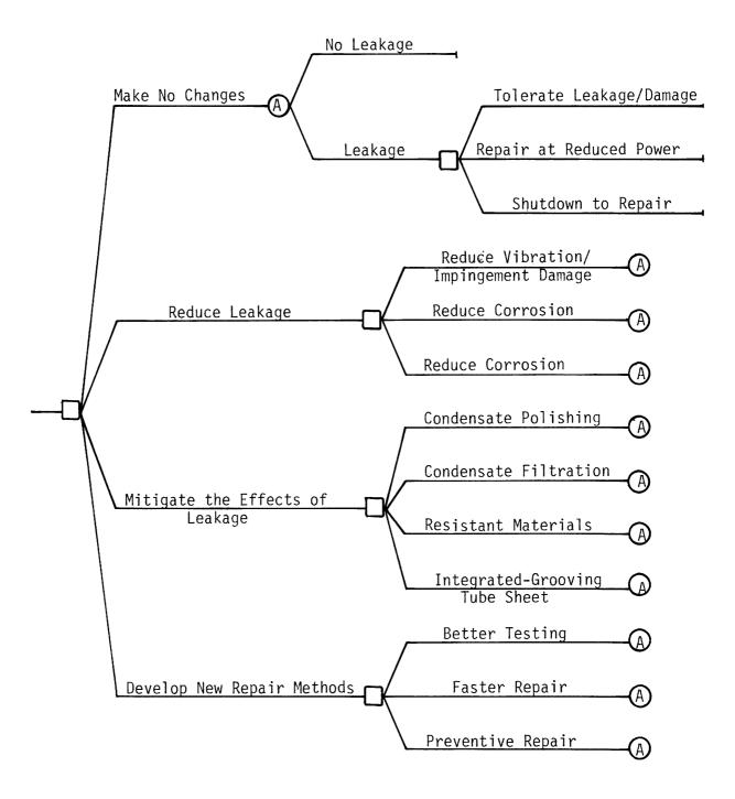
Figure 2. Simplified Tree for Condenser Outage Problems
