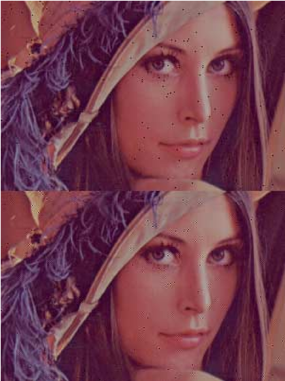
Figure 5-11: Simulated video display with missing pixels; uncorrected (top), and corrected using proposed algorithm (bottom). A viewing distance of five feet is recommended.
