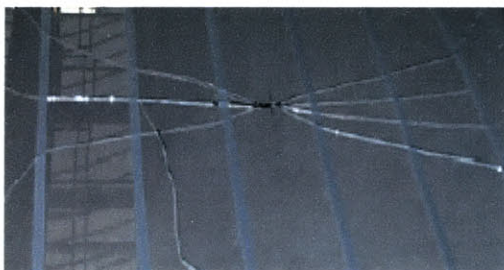
Figure 13: Typical crack pattern of heat-strengthened glass [20]
