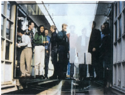
Figure 22: a) Loading test on completed bridge using employees from Kraayvanger Urbis, b) Looking upward into completed footbridge [38]
