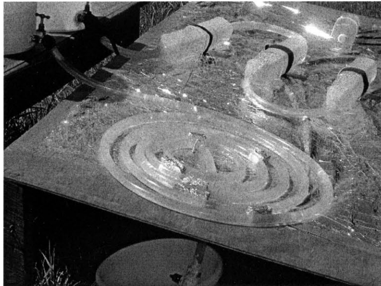
Figure 4.2: The three solar disinfection systems assembled. The modified SC-SODIS (middle) was not broken at the time of this photograph, but was eventually discarded due to structural failure.
