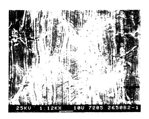
Figure 6.103 The Scanning Electron Micrographs for the Tensile Specimen of The HTMA Condition of Heat NX2650 Tested at a Strain Rate of  $2.2 \times 10^{-4} \, \mathrm{sec}^{-1}$  at 320 C (upper fracture surface lower side wall).
