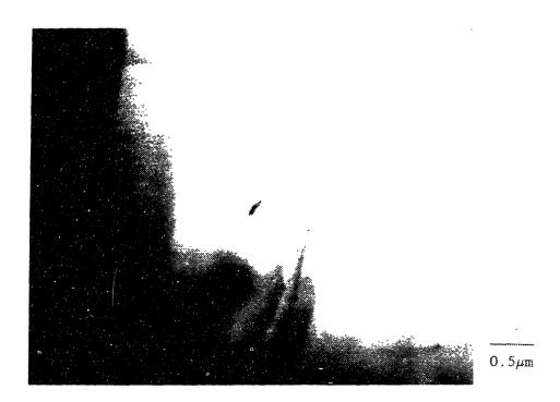
Figure 6.16 The STEM Micorgraphs for a 2.2cm Diameter Tubing of a HTMA Condition of Heat 96834 (upper micrograph at inner diameter region and lower at outer diameter region).
