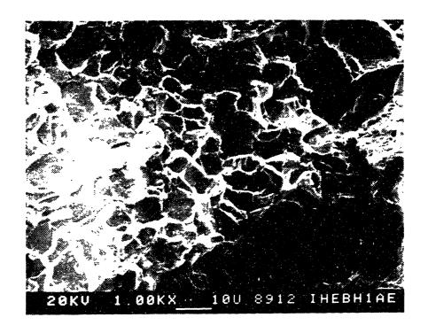
Figure 6.70 Fracture Surface of the AES Specimen for the EBH Condition of an Alloy X-750 Heat 96457E6.
