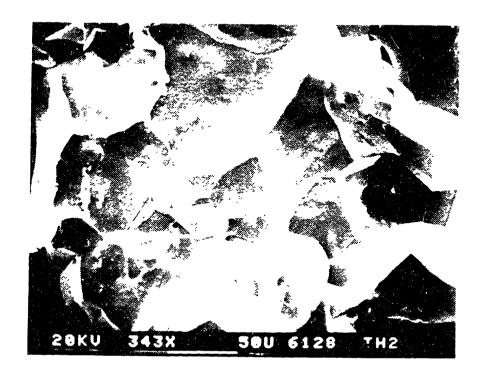
Figure 6.67 Fracture Surface of the AES Specimen for the AHTH Condition of an Alloy X-750 Heat 96457E6.
