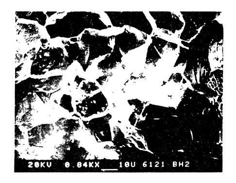
Figure 6.66 Fracture Surface of the AES Specimen for the BH Condition of an Alloy X-750 Heat 96457E6.
