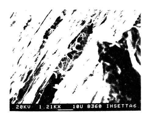
Figure 6.134 The SEM Fractographs of the AH Condition after the SETT in a 0.05M  $\rm Na_2SO_4$  (pH=3) Solution with a Strain Rate of  $\rm 6.7x10^{-5}~sec^{-1}$  and a Potential of -450 mV(SHE).
