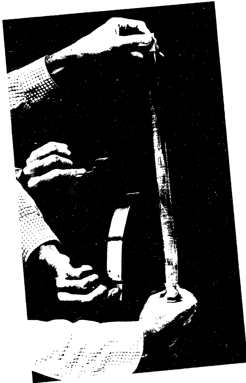
Figure 14. Multiple exposure photograph of flexible 2.5 cm wide ESR ribbon. The ribbon is approximately 90 microns thick.
