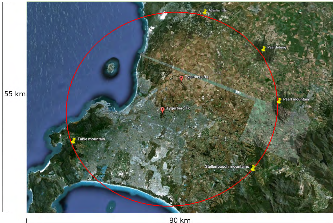
Figure 4.4: The Tygerberg receive site has good aspect of the predominant flight path to the North-East but it suffers from severe multipath effects at 60 km bistatic range due to many large terrain structures lying at this range as shown by the red ellipse and thumbtacks.
