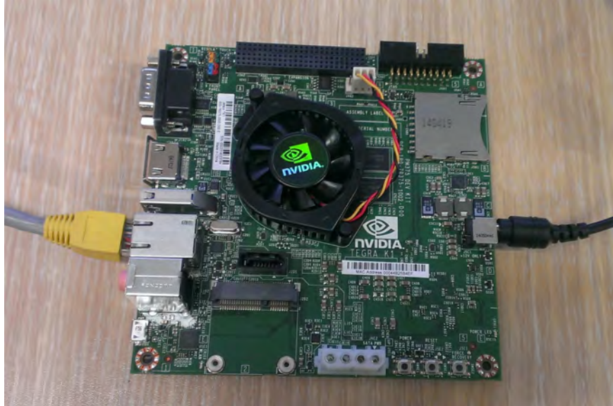
Figure 3.15: NVIDIA Jetson TK1 development kit.
