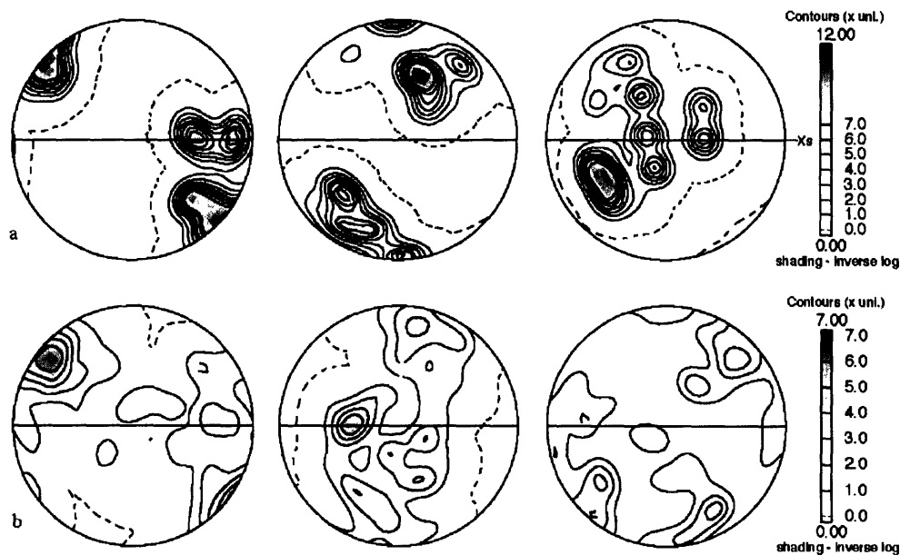
Figure 6: Variation in LPO for populations of different grain sizes from the same rocks. Samples shown here are from the 25 m wide dunite. a) Grains larger than 3 mm (N=41) exhibit a clear orthorhombic (010)[100] LPO. b) In contrast, grain smaller than 3 mm (N=114) record a girdled \{0kl\} [100] LPO.
