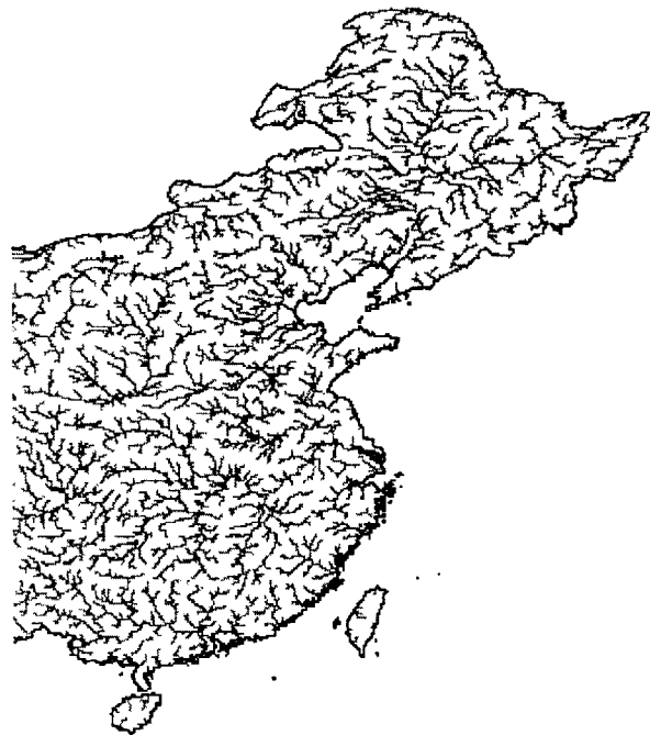
Figure 3-4: Vector stream network of eastern China derived with a stream threshold value of 1000.
