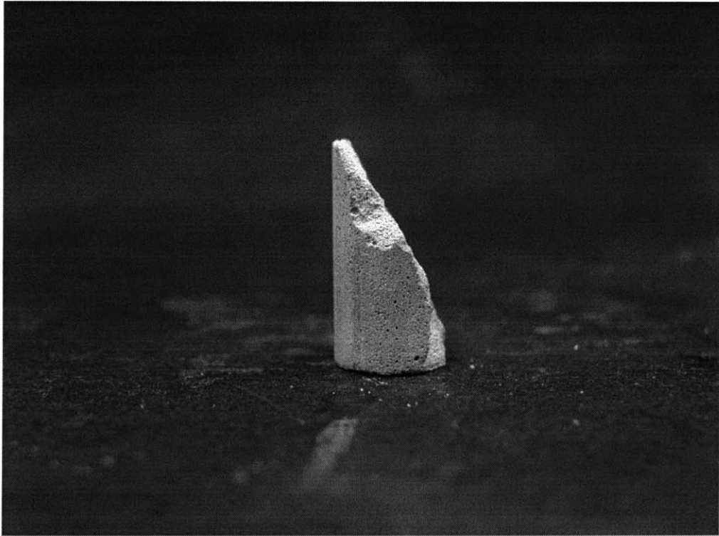
Figure 6-9: Typical leached cement paste specimen fragment after failure on the shear plane.
