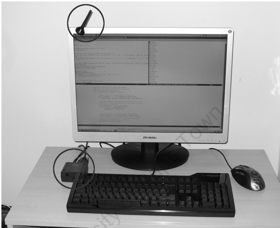
Figure 4.2: Workstation showing Siemens TC35i and aerial (circled).
