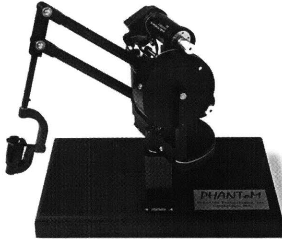
Figure 1.1 Force-Feedback Devices for augmenting on-screen objects. a) Immersion's Impulse Engine b) SensAble's PHANTOM
