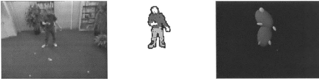
Figure 2-1: The PFINDER system extracts regions using hierarchical clustering based on color classification and models these regions as blobs. The left image depicts a typical video image, the center depicts the clustered regions, and the right depicts the computed 2-D blob features.
