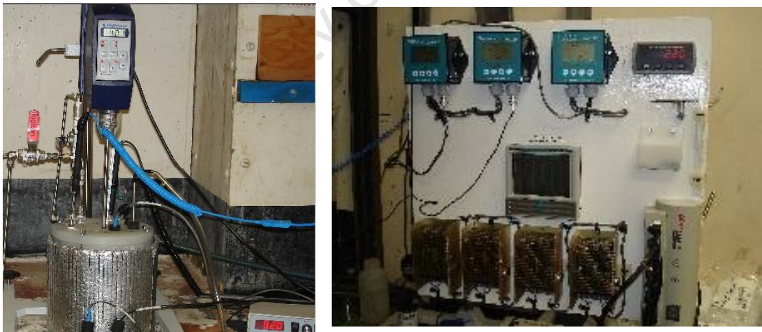
Figure 3. 2: Actual Reduction Releach Reactor (a) and Controls (b)
