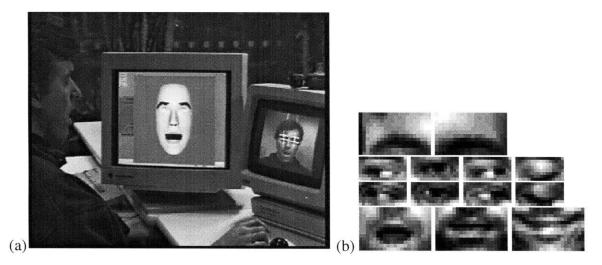
Figure 3-4: (a) Overview shot of full system for tracking facial expression in real-time. User is on left, vision system and camera is on right, and animated face is in the center of the scene. The animated face matches the state of the users face in real-time, including eye-blinks (as is the case in this shot.) (b) Spatial view models learned by unsupervised clustering method for region-based face mimicking example; independent view models were found for eyes, eye-brows, and mouth regions.
