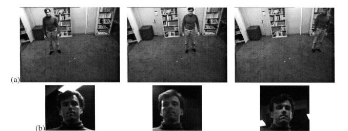
Figure 4-2: Active tracking in an interactive room; images acquired from (a) wide and (b) narrow field of view cameras as user moved across scene and narrow camera tracks head.
