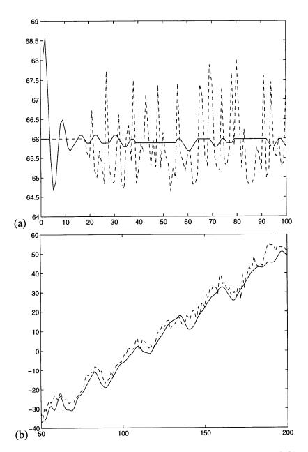
Figure 4-7: Tracking results: plot of pan angle for (a) stationary user, and (b) moving user who walked across room while oscillating head. Dashed line shows pan position under open-loop control; solid line shows pan position under closed-loop control.
