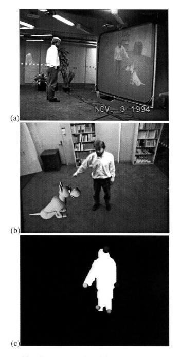
Figure 2-2: Person tracking in a system for vision-based interaction with a virtual environment. (a,b) A user sees him/herself in a "magic mirror", composited in a virtual environment. Computer vision routines analyze the image of the person to allow him/her to effect the virtual world through direct manipulation and/or gestural commands. (c) Results of feature tracking routine; head, hands, and feet are marked with color-coded balls.
