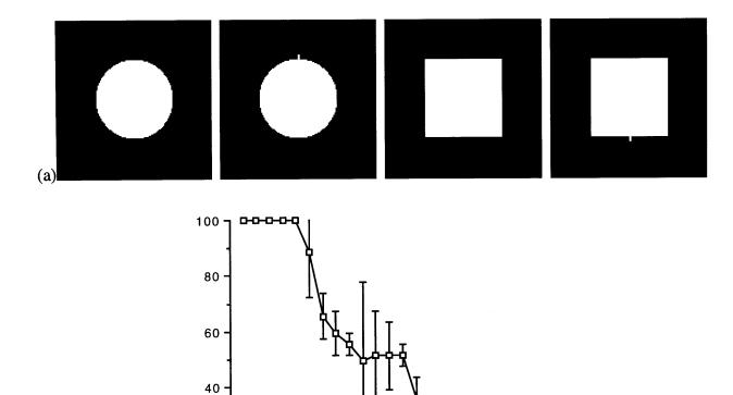
(b) 0 20 40 60 80 100 Figure 5-3: AGR results for simple imagery targets: (a) set of four target patterns, where the first and last pair are indistinguishable at low-resolution (b) recognition performance (percentage of correct trials) for varying amounts of observation noise.
