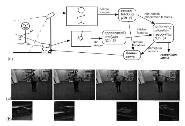
Figure 5-2: Four gesture patterns in interactive interface domain which require foveated images for discrimination. (a) Overview of AGR system in interactive domain; active camera tracks the relevant hand to identify the gesture, as described in text. (b) Output from wide field of view camera; (c) output from narrow field-of-view active camera.
