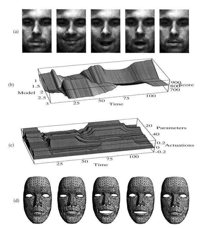
Figure 3-3: Interactive facial expression tracking in real time. A set of normalized correlation view models are used to characterize facial state, and then used to interpolate a set of motor control parameters for a physically based face model. View models are acquired using unsupervised clustering while the interpolation is trained using supervised learning. See text for details.
