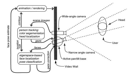
Figure 4-1: Overview of system for face/body tracking and pose estimation, Objects are rendered on Video Wall and react to facial pose or expression of user. Static, wide-field-of-view, camera tracks user's head, and drives gaze control of active, narrow-field-of-view camera. Appearance/view-based analysis is run on face images from active camera, to provide pose or expression estimates for objects/agents to react to, and to provide closed loop face tracking feedback for active camera.
