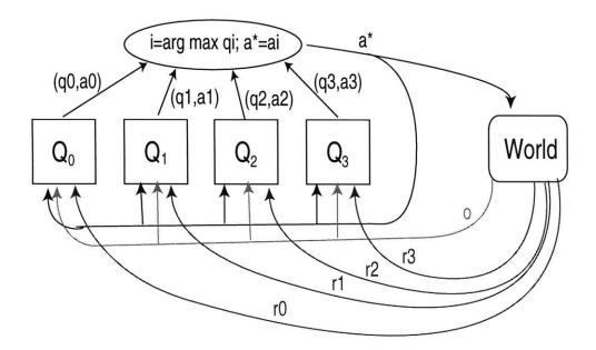
Figure 5-7: Multiple model Q-learning: one Q-learning agent for each target gesture to be recognized, with coupled observation and action but separate reward and Q-value.
