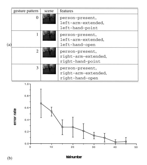
Figure 5-4: Simple target performance with random exploration (a) set of targets which can be discriminated using a single foveated observation. For each run, one gesture was randomly chosen as target, and the other three used as distractors. (b) results averaged over 100 runs; error rate is plotted as a function of trial number (proportional to timestep). Random exploration is sufficient to learn a recognition policy in these cases.
