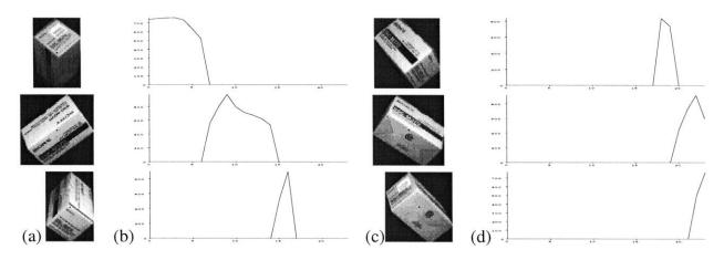
Figure 3-2: (a,c) Spatial view models automatically acquired from a sequence of images of a rotating box. (b,d) Normalized correlation scores for each model as a function of angle.
