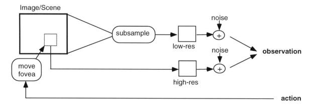
Figure 5-1: Formulation of AGR task with simple static images as world state.
