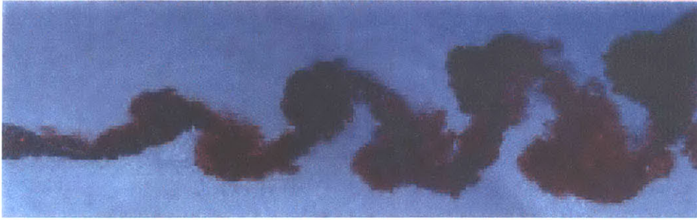
Figure 1-1: Dye visualization of the MIT RoboTunawake showing a reverse Kármán wake pattern. (from [53])
