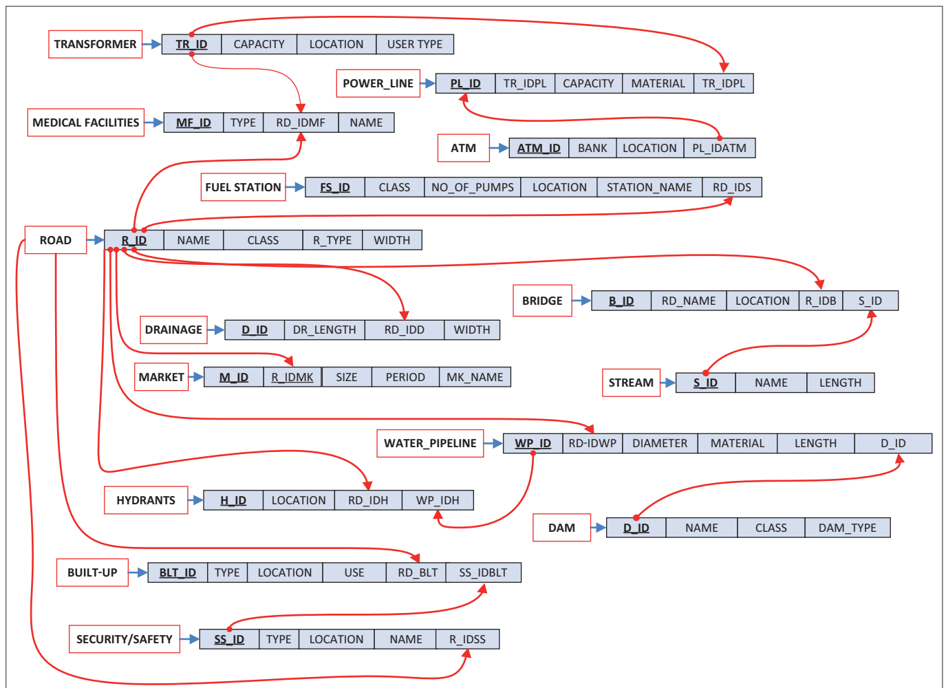
FIGURE 5: Logical model designed for urban critical infrastructure and disaster management.
