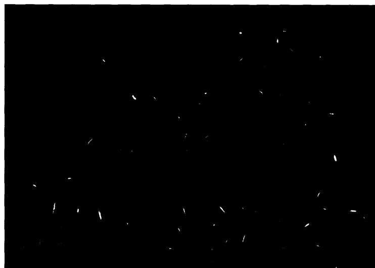
Figure 6-3: Fluorescent microscope image of \text{Alq}_3 crystals grown at 0.05 Torr
