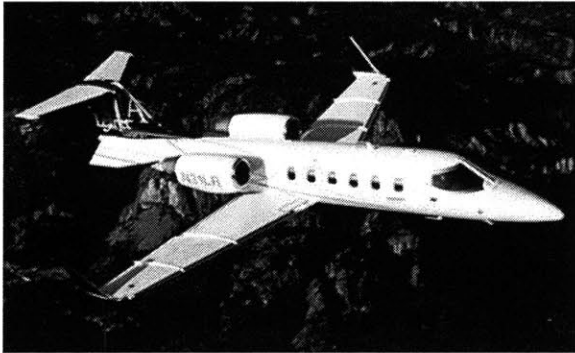
Figure 47: Typical Aft-Mounted, Twin-Engine Business Turbofan (Lear 31)
