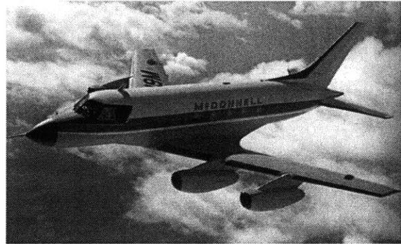
Figure 48: Early Business Jet Prototype with Wing-Mounted Engines (McDonnell 119)
