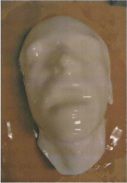
fig.32 3d printed face with silicon moulded skin on top.
