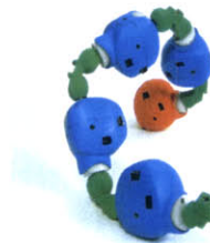
actives connected with tetrahedrals and programmed with a queen create a spring-like helix
