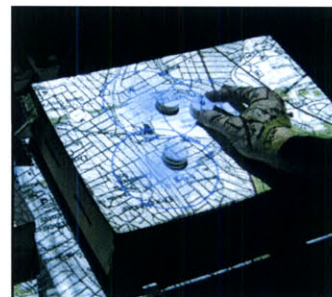
Actuated Workbench, Pangaro, 2002 - uses an array of electromagnets to move objects on a table top
