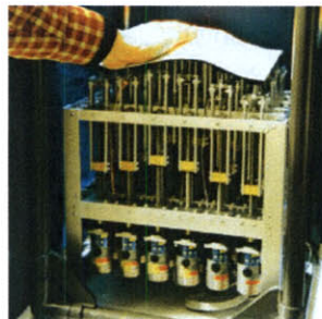
Feelex, Iwata, 2001 - uses an array of mechanical actuators to change the topography of the flexible membrane surface
