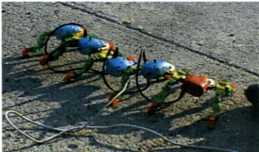
sending a delay through this “cat-erpillar” causes it to move with a wave-like motion
