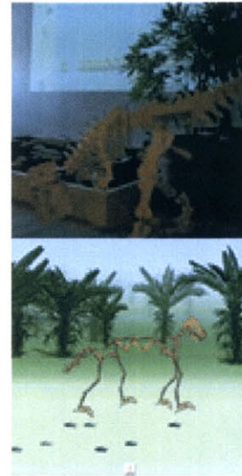
Dino Stable, Strohecker, 2003 - physical model (top) is tagged to be sensed as part of on-screen creation (bottom)
