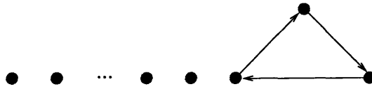
Figure 6-3: This graph demonstrates the worst integrality gap that we are aware of for the semidefinite programming relaxation for the linear ordering problem ( P ). For a 3-cycle with five isolated vertices, the gap is about 2.25.
