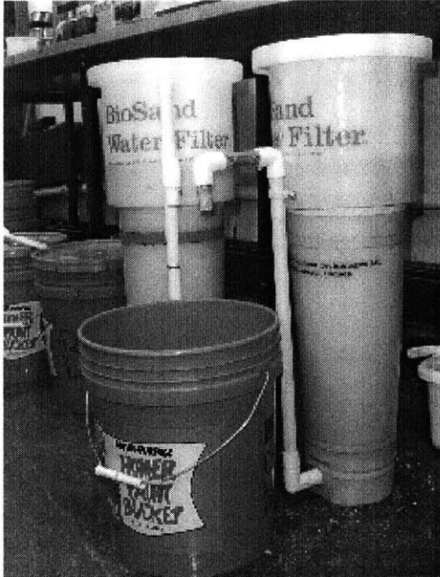
Figure 9.2: BioSand filters setup during laboratory experimentation.
