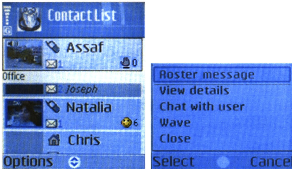
Figure 2-2: The Contact List Screen (on left) provides availability information. The options menu for this screen is on the right.
