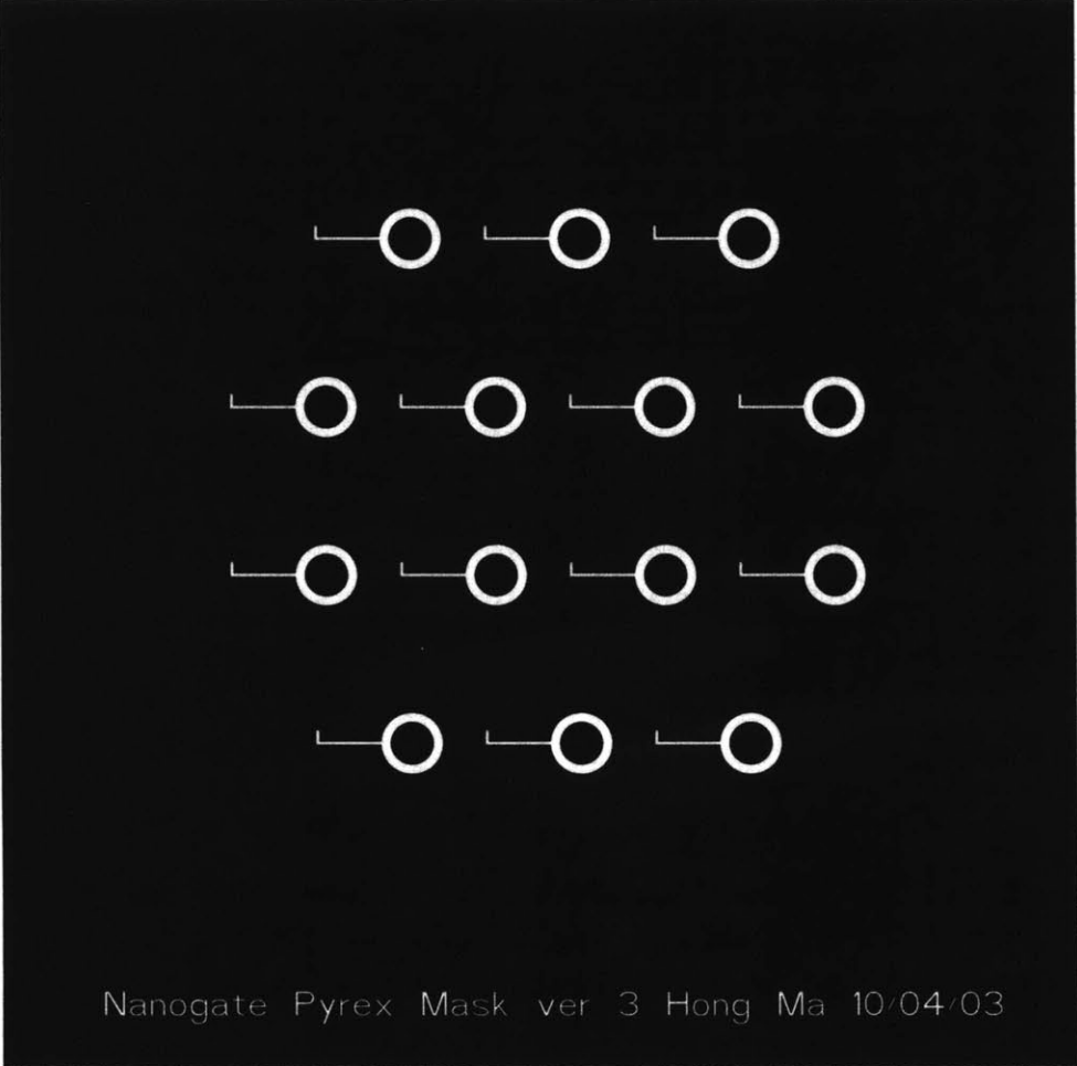
Figure 37: Mask for the Nanogate Pyrex base
