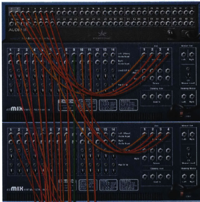
Figure 78. The back side of two eight-channel mixers in Reason that are coupled to send eight channels of audio to any of the Beatbugs through the MOTU audio interface.
