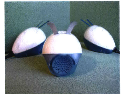
Figure 44. The Beatbugs design. Two bend-sensors antennae and a velocity-sensitive drum trigger allow for entering and manipulating rhythmic motifs
