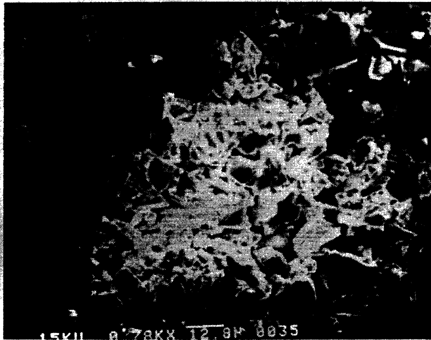
Figure 16 - Crystalline Structures in ARM-1 Glass with 10% ThO 2
