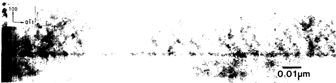
4.3 (b) XTEM micrograph of epitaxial film, cleaned in-situ at 600°C for 20 minutes.
