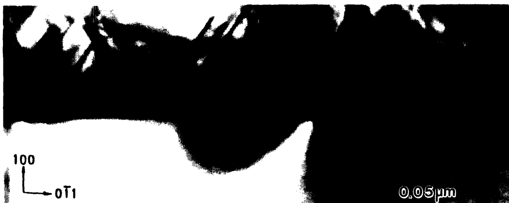
4.2 (b) XTEM micrograph of epitaxial film, cleaned in-situ at 600°C with DC bias set at -50V
