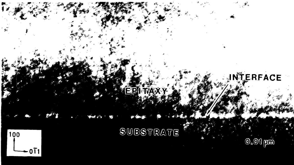
4.3 (c) HRXTEM micrograph of epitaxial film, cleaned in-situ at 600°C for 20 minutes.
