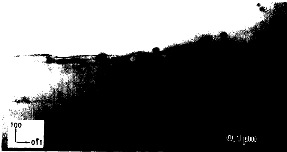
4.3 (a) XTEM micrograph of epitaxial film, cleaned in-situ at 600°C for 2 minutes.
