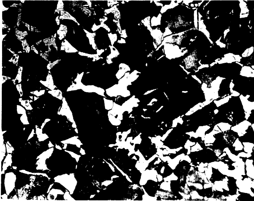
Fig. 3.2 The used Class L microstructure. Micrograph taken from Gleeble specimen 593-3, deformed at 1100°F to 3.4% total strain taken from area A of Fig. 2.6 at a magnification of 400x (abbreviated format: 593-3, 1100°F, 3.4%e, A, 400x).
