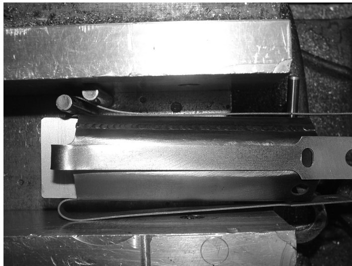
Figure 4.14 Formation of Primary Bends in Tabs
