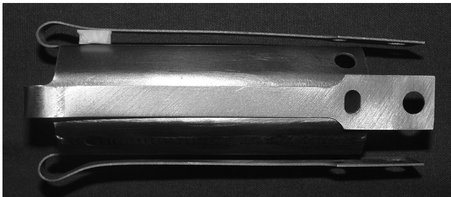
Figure 4.16 Reversal of Springback into Preload
