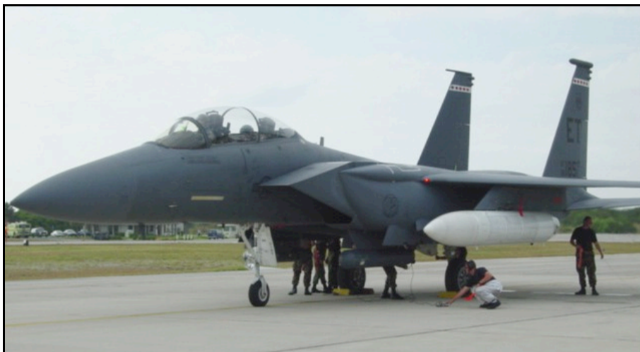
Figure 6-9 The EGT-Pod and its carrying vehicle (Courtesy of Chris Anderson)
