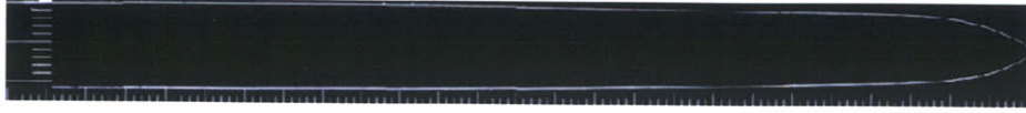
Figure 4-4: Phase contrast image of a stainless steel needle with R_{Rod} = 0.54 mm with a tapering tip. The needle becomes a uniform thickness beyond 6mm from the tip. The smallest gradation in the ruler is 0.1mm.
