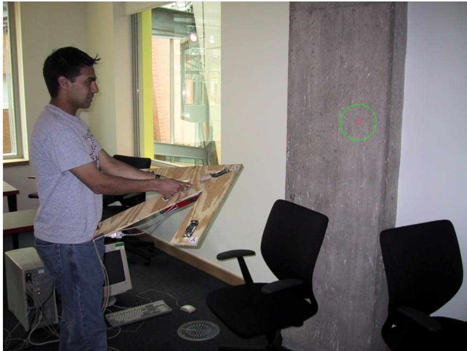
Figure 3-9: A user marks a wall vertex using the frame and range finder. The range finder projects a red spot on the wall (shown here circled in green), which indicates to the user which feature s/he is about to mark.
