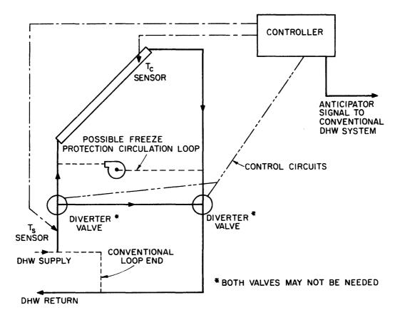
Fig. 3. Design Concept--Solar Assisted Domestic Hot Water
