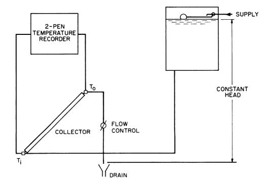
FIG. 5. EQUIPMENT FOR SITE OR COLLECTOR EVALUATION
