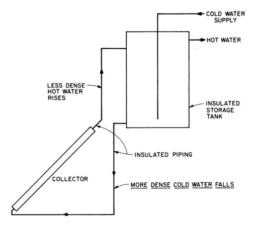
FIG. 4. THERMOSYPHON CIRCULATION SYSTEM
