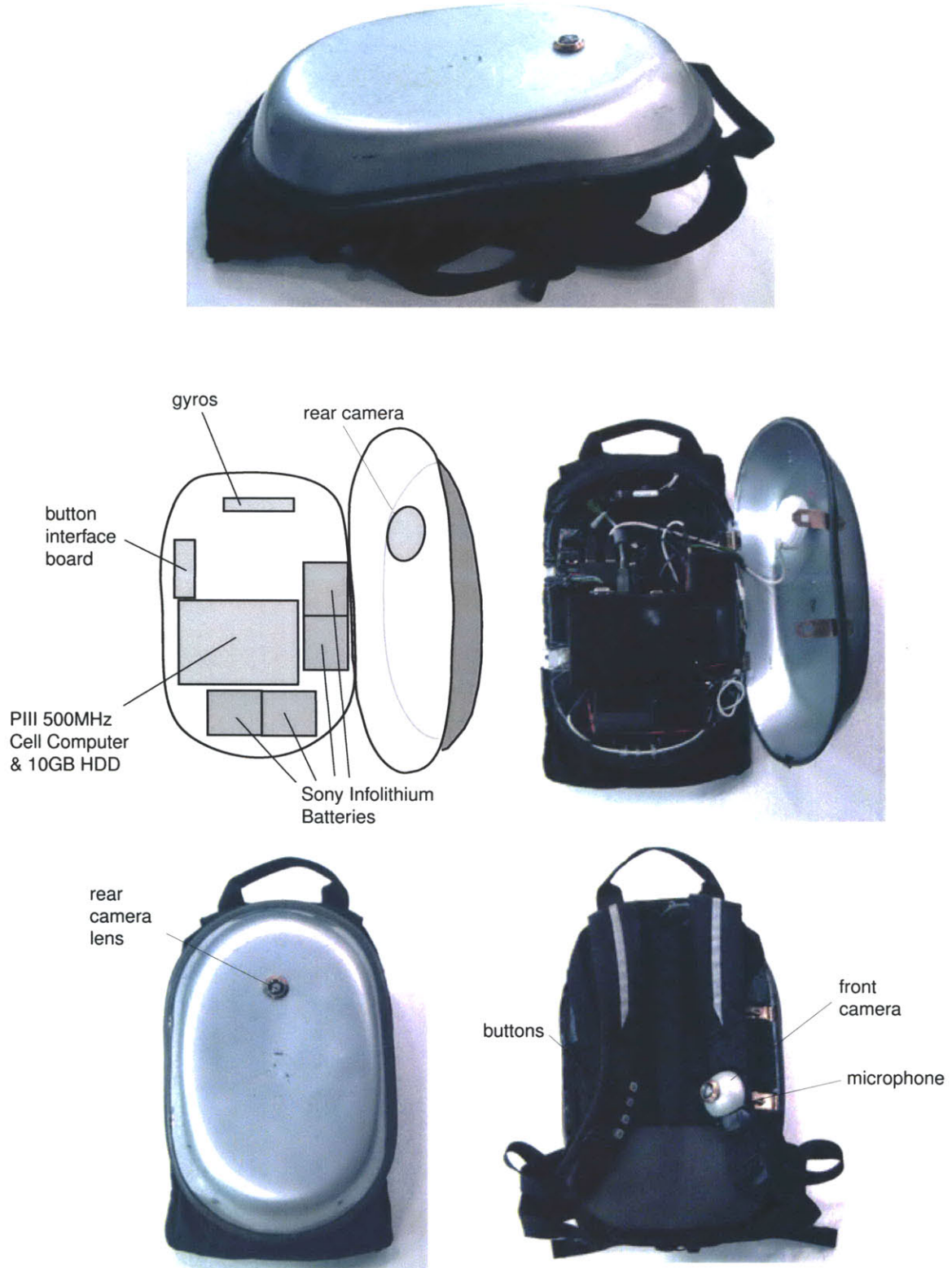
Figure 4-4: The Data Collection Wearable Schematic
