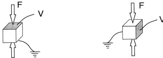
Figure 2-1: Axial test configurations: (a) longitudinal test and (b) transverse test.
