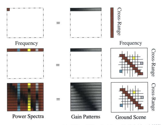
Figure 3.11 Matrix Representation of the PSF Scan Within a Single Range Bin [Sedwick et al, 2000]
