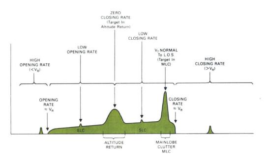
Figure 2.14 Clutter Spectrum for a Forward-Looking Radar [Stimson, 1998]
