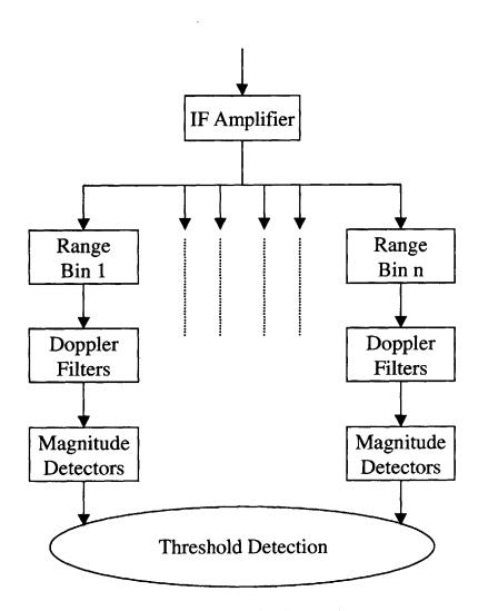
Figure 2.7 Block Diagram for Radar Signal Processing
