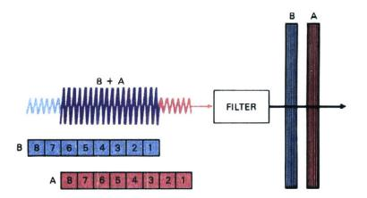
Figure 2.13 Improved Range Resolution from Pulse Compression [Stimson, 1998]
