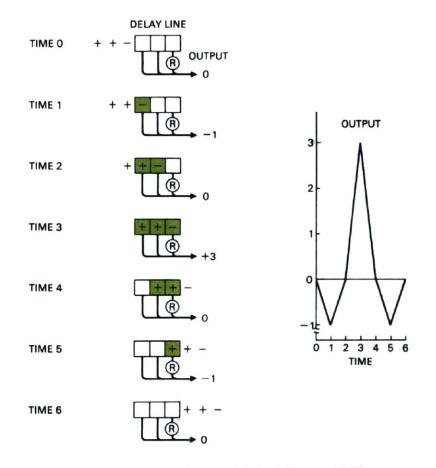
Figure 2.12 Illustration of Binary Phase Modulation [Stimson, 1998]
