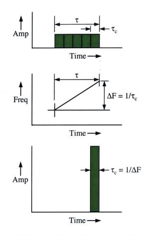
Figure 2.11 Compressed Pulse in Linear Frequency Modulation
