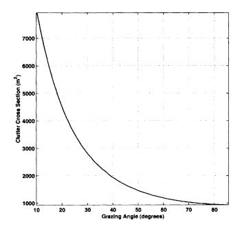
Figure 4.5 Clutter Cross Section as a Function of Grazing Angle
