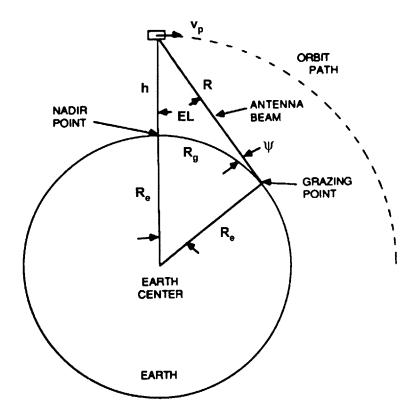
Figure 4.8 Radar-Earth Geometry [Cantafio, 1989]
