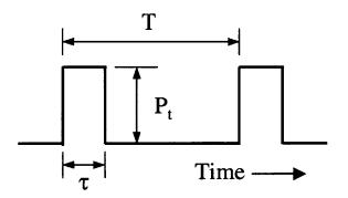
Figure 2.5 Parameters of a Pulsed Waveform
