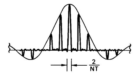
Figure 2.6 Pulsed Signal Spectrum [Stimson, 1998]
