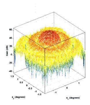
Figure 4.3 Example Point Spread Function of a Sparse Aperture Interferometer
