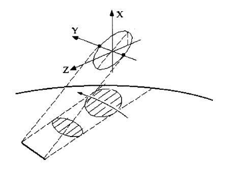
Figure 3.2 Free Orbit Solution to Hill's Equations
