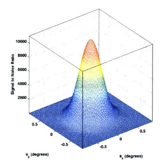
Figure 4.6 Footprint Variations in the Signal-to-Noise Ratio
