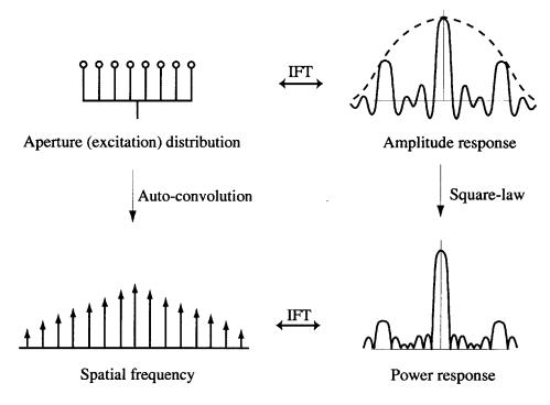
Figure 3.6 Aperture Synthesis with a One-Dimensional Array [Shaw, 1998]
