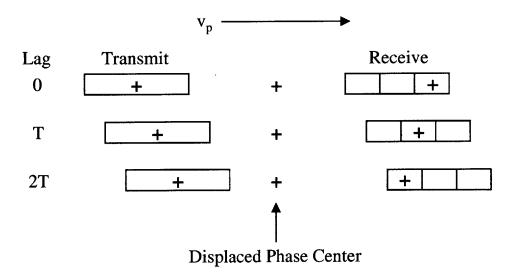
Figure 3.8 Three-Pulse DPCA Cycle
