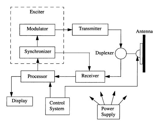
Figure 2.2 Common Elements of a Radar System
