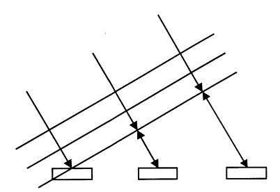
Figure 3.7 Array Steering With Time Delays
