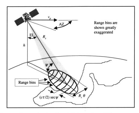
Figure 2.1 Geometry for a Space-Based Radar System [Shaw, 1998]
