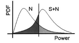
Figure 2.10 Statistical Representation of the Signal and Noise Power Returns
