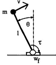
Figure 8-3: Simple pendulum model of the dynamics of the 3d simulation in the frontal plane. The robot mass,  $m$  is lumped at a point. The leg is of length  $l$  at an angle  $\theta$  from vertical. The foot has a half width of  $w_f$ , with torque  $\tau$  being applied at the ankle. This model is useful for studying the effects of foot placement and ankle torque on lateral velocity.
