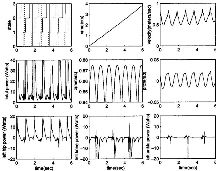
Figure 5-6: **[SIM]** Planar simulation data exploiting natural dynamics. The first row contains, left to right, state of the legs, forward distance traveled, and forward velocity. The second row contains total power, body height, and body pitch. The last row contains joint power at the hip, knee, and ankle of the left leg.
