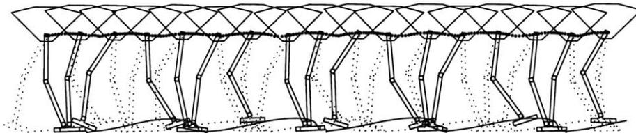
Figure 4-5: **REAL** Elapsed time snapshot of the Spring Flamingo walking data in Figure 6. The drawings of the robot are spaced approximately 0.5 seconds apart. The left leg is dotted while the right leg is solid. Lines show the path of the tips of the feet and the hip trajectory. The robot walks from left to right.
