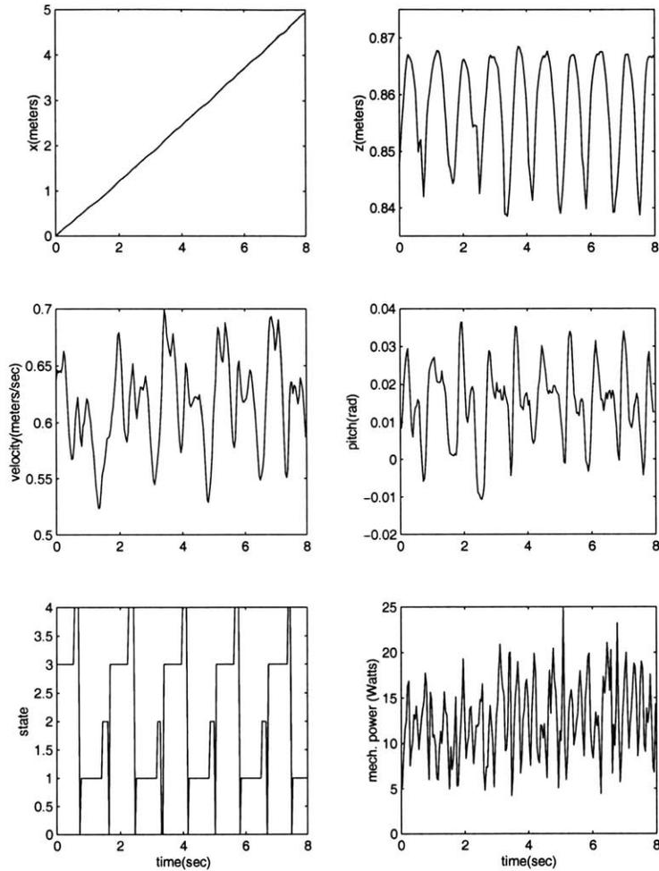
Figure 4-4: **REAL** Spring Flamingo walking data. Left graphs display, from top to bottom the horizontal position ( $x$ ) and horizontal velocity of the body and the state of the state machine. Right graphs display the vertical position ( $z$ ) and pitch ( $\theta$ ) of the body and mechanical power being applied to the joints.
