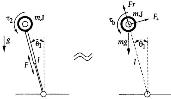
Figure 3-8: Inverted pendulum with flywheel and linear actuator (left). Free body diagram (right) showing external force and torque equivalents. The two systems are dynamically equivalent if  $F_{\perp} = \frac{\tau_1^2}{l}$ ,  $F_r = F$ , and  $\tau_b = \tau_2$ .
