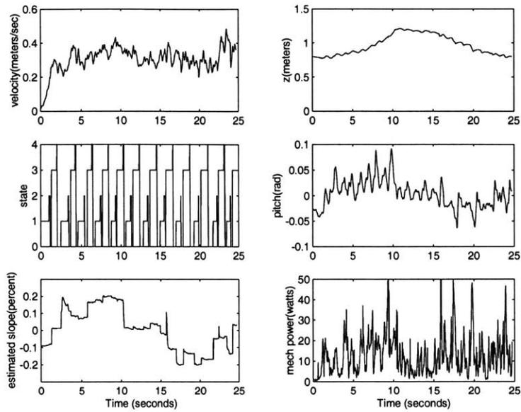
Figure 4-8: **REAL** Spring Flamingo walking data while walking over a 15° ramp.
