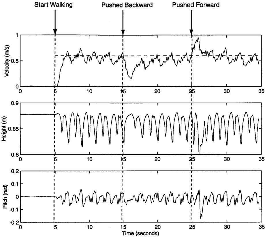
Figure 7-6: **REAL** Data showing disturbance rejection due to being pushed. The robot is pushed backward at approximately 15 seconds which decreases its speed and pushed forward at approximately 25 seconds which increases its speed. In both cases, the robot regains the desired speed of approximately  $0.6 \frac{m}{s}$ . The second push creates a significant disturbance in both height and pitch, yet the robot quickly recovers.
