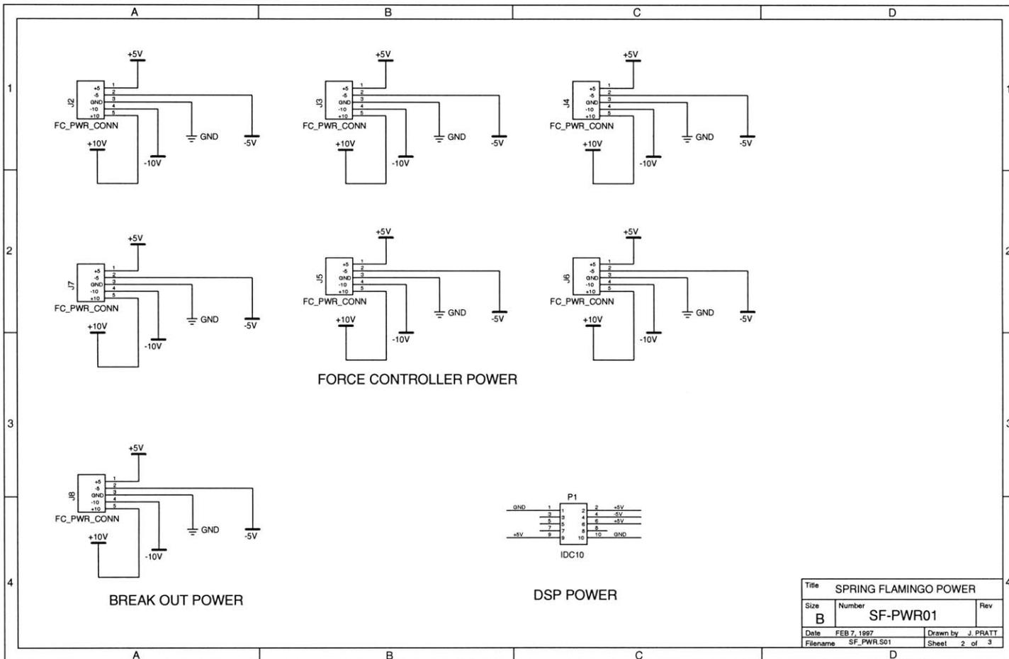
Figure A-24: Power Board Schematic Page 2 of 2.
