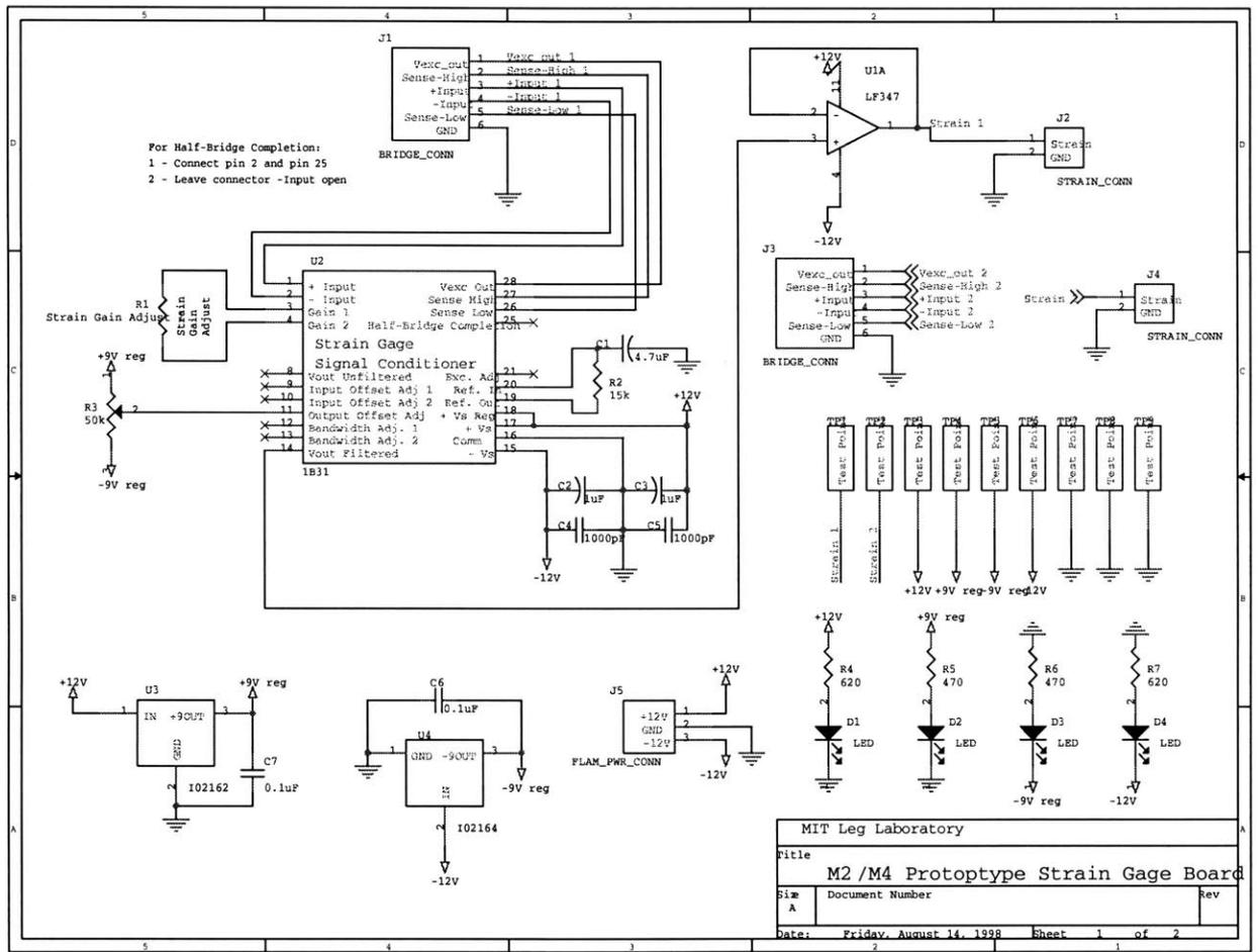
Figure A-27: Strain Gage Conditioning Board Schematic Page 1 of 2.
