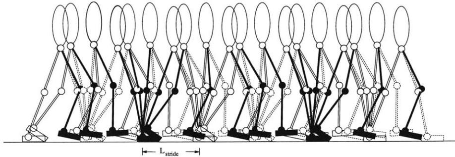
Figure 6-6: Cartoon of human walking with three legs. Two full walking cycles are shown.  $L_{stride}$  is the stride length. With three-legged walking swing-time is limited to twice the stride time. Therefore, if minimum swing-time is a limitation of human walking, a three-legged human should be able to walk twice as fast as a two-legged human.
