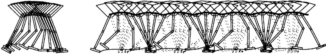
Figure 7-4: **REAL** Elapsed time snapshot of Spring Flamingo walking at  $1.1 \frac{m}{s}$ . The drawings on the left are spaced approximately 0.06 seconds apart and show the swing phase of one leg. The drawings on the right are spaced approximately 0.2 seconds apart. The robot walks from left to right. Snapshots of this data spaced approximately 0.06 seconds apart are also plotted on the bottom of this thesis.
