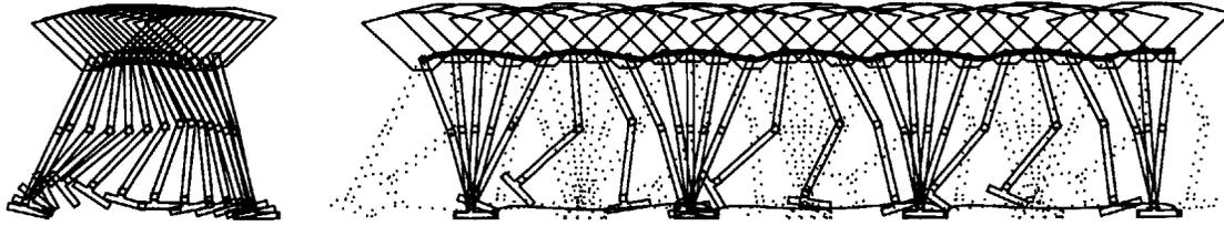
Figure 5-5: **[SIM]** Elapsed time snapshot of the simulated robot walking data. The drawings on the left are spaced approximately 0.08 seconds apart and show the swing phase of one leg. The drawings on the right are spaced approximately 0.25 seconds apart. The right leg is dotted while the left leg is solid. Lines show the path of the tips of the feet and the hip trajectory. The robot walks from left to right at approximately  $0.8 \frac{m}{s}$ .
