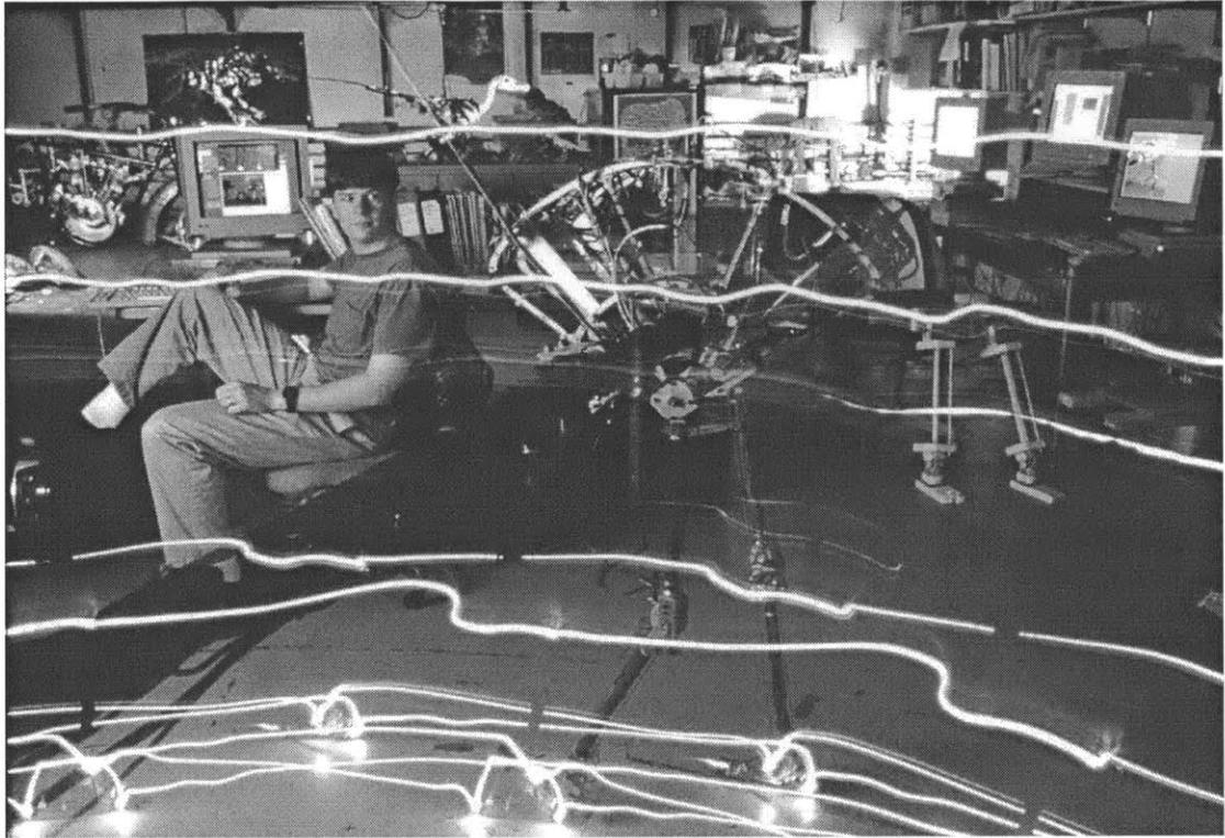
Figure 1-1: Spring Flamingo taking a stroll with the author looking on. Lights trace out the motion of the top and middle of the robot's body, the hip, knee, and ankle joints, and the toe and heel of the feet. Photo by Peter Menzel, Copyright 1999. Reproduced with permission.
