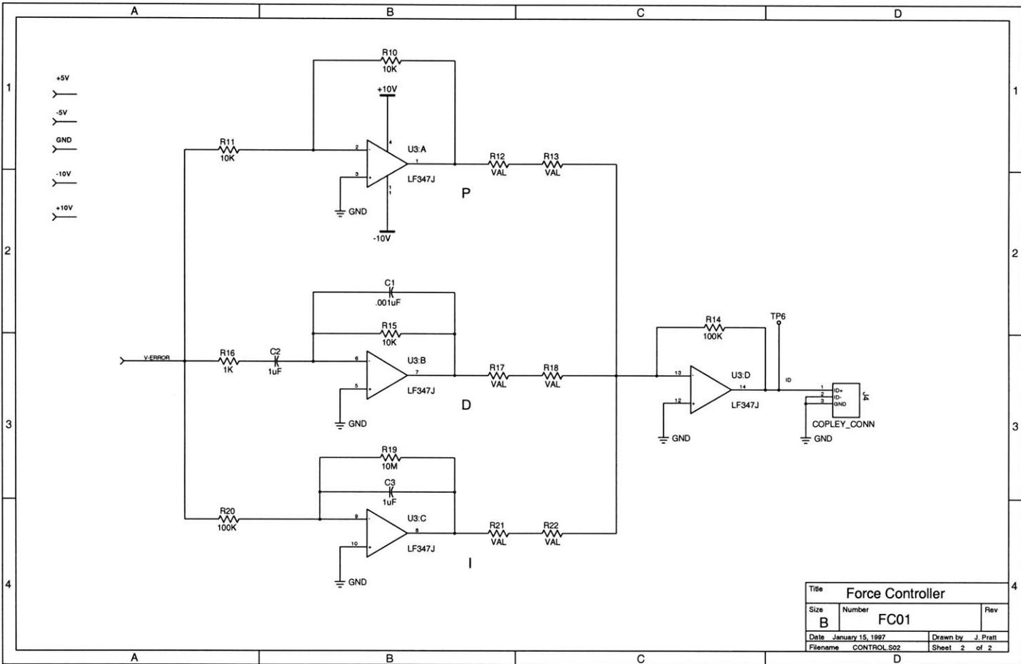
Figure A-26: Force Control Board Schematic Page 2 of 2.
