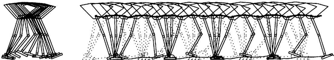
Figure 5-9: **REAL** Elapsed time snapshot of the physical robot walking data exploiting natural dynamics. The drawings on the left are spaced approximately 0.07 seconds apart and show the swing phase of one leg. The drawings on the right are spaced approximately 0.4 seconds apart. The robot walks from left to right at approximately  $0.5 \frac{m}{s}$ .
