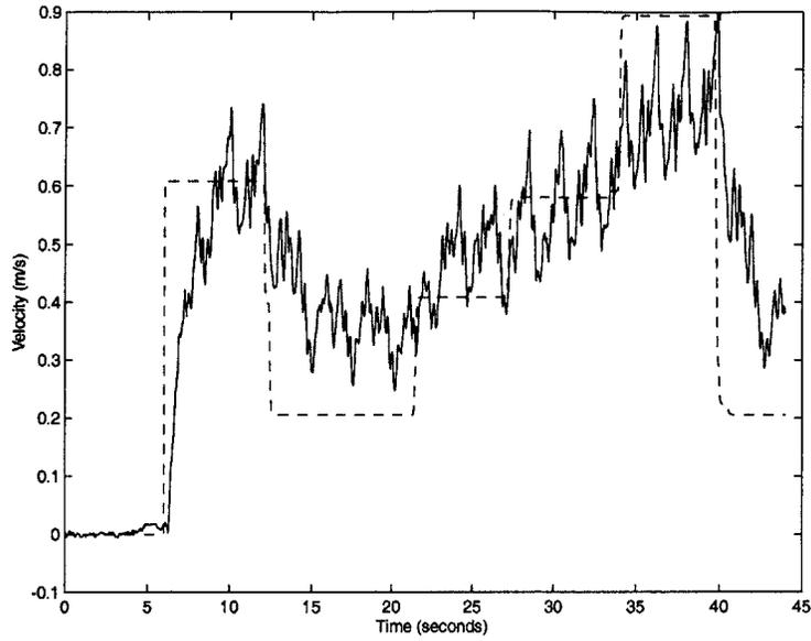
Figure 7-5: **REAL** Data showing control of walking speed. The actual speed (solid) follows the trend of the desired speed (dashed), although it does not track it exactly. The robot is standing and balancing for the first five seconds.
