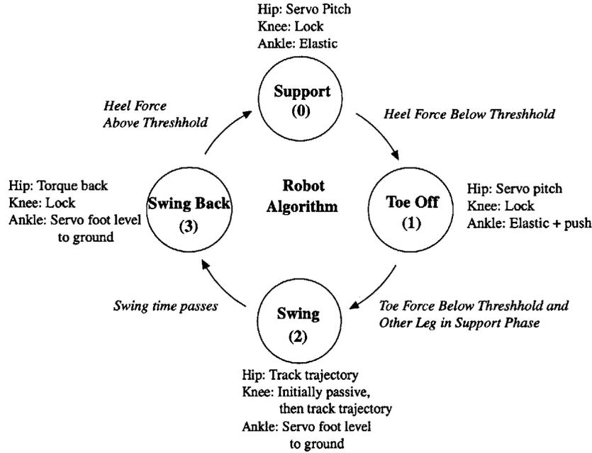
Figure 7-1: **REAL** Fast walking algorithm. Each leg has a state machine which is in one of four states. State transition conditions and actions in each state are shown.
