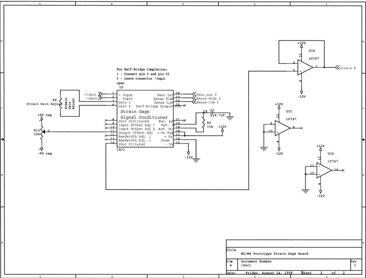
Figure A-28: Strain Gage Conditioning Board Schematic Page 2 of 2.
