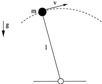
Figure 6-4: Rotating pendulum model for estimating walking speed limit. Centrifugal force of  $\frac{mv^2}{l}$  will equal the gravity force of  $mg$  at the top of the arc if  $v^2 = gl$  (Froude Number equals 1.0). At that speed the force on the foot will fall to zero.
