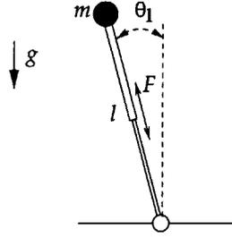
Figure 3-4: Simple inverted pendulum with linear actuator. The rotational dynamics are independent of the actuator force and only depend on  $g$ ,  $l$ , and  $\theta_1$ .
