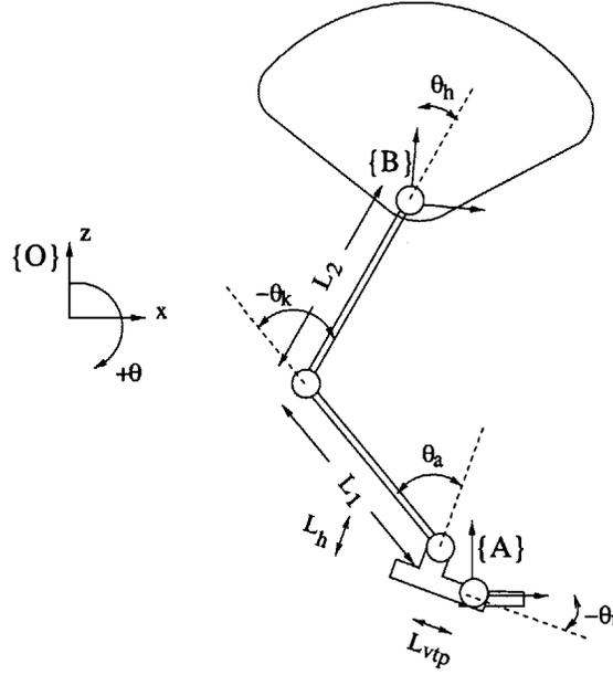
Figure 4-1: Virtual Model implementation on a single leg. Reaction frame  $\{A\}$  is assumed to be in the same orientation as reference frame  $\{O\}$  so that  ${}^O_A R = I$ . For this derivation, we assume the robot is in the configuration with the knee bent backward. However, the resulting equations hold whether the knee is bent backward or forward.
