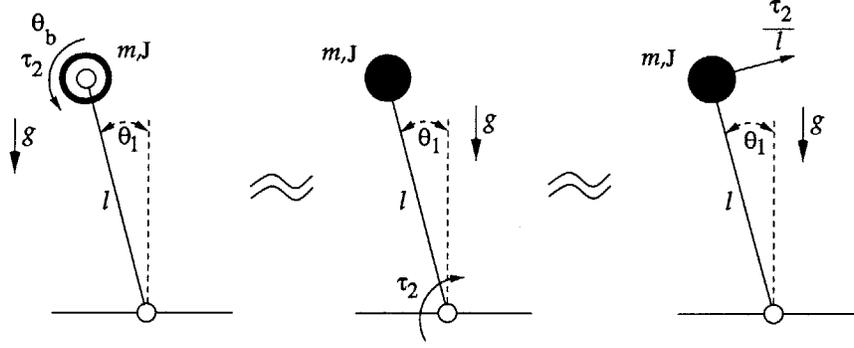
Figure 3-7: Inverted pendulum model with flywheel of mass  $m$  and inertia  $J$  (left). Applying a torque of  $\tau_2$  on the flywheel is equivalent to applying an ankle torque of  $\tau_2$  on the model in the middle or an external force of  $\frac{\tau_2}{l}$  on the model on the right.
