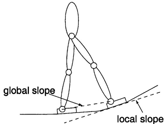
Figure 4-6: Graphical definition of global slope and local slope. In general, the global and local slopes will be different. The global slope may be a better estimate, but the local slope has predictive qualities for smoothly rolling terrain.
