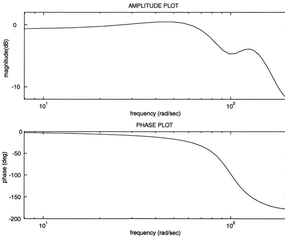
Figure A-10: Experimentally determined bode diagram of actuator force response. The -3dB magnitude cross-over point is at approximately  $90 \frac{rad}{s}$  (14Hz).
