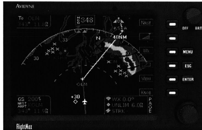
Figure 2.2: Avidyne FlightMax 750 Multi-Function Display (MFD)
