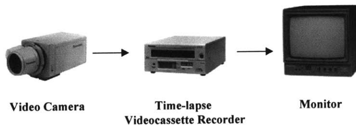
Figure 2-1: A typical security camera system. The video signal is taken from a video camera typically mounted on a wall or ceiling and recorded with a time-lapse videocassette recorder. The recorded tape can then be viewed later on a monitor.
