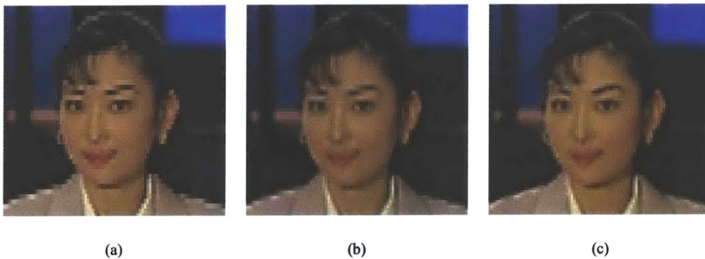
Figure 6-9: (a) Line repetition. (b) Linear interpolation. (c) Martinez –Lim algorithm.
