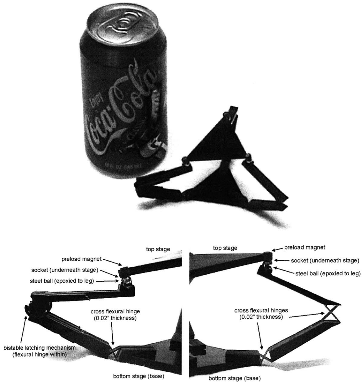
Figure 3.10. Test prototype of an unactuated single BRAID stage.
