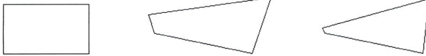
Figure 9.25 Illustrating the possible evolution of a rectangular plan if wall widths are used as variables. In the left image, one of the walls is tending to zero, turning the plan into a triangle.
