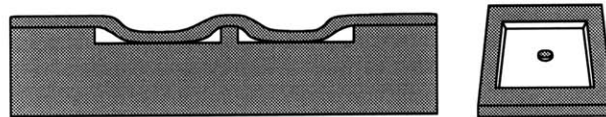
Figure 4-29: Plate from wafer 4 (LOCOS:oxide+nitride), square plate with central pedestal, side= 1772\mu\text{m} , h=11\mu\text{m} , L=2\mu\text{m} , P_{CAV}=\text{vacuum} . b) Plate geometry.
