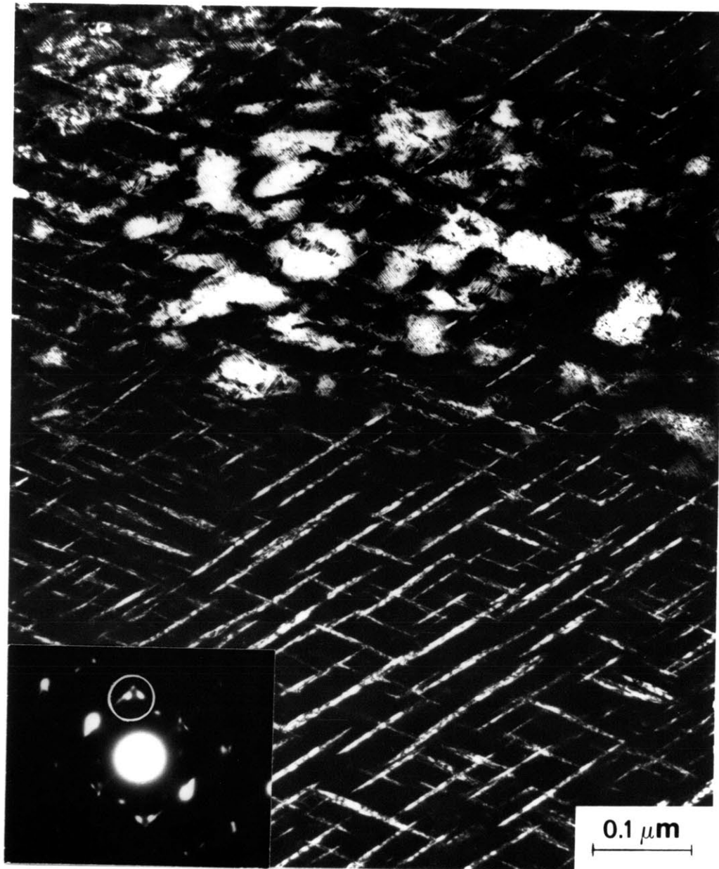
Figure 8-4. Dark-field micrograph of the same crystal as in Figure 8-3, but after slight tilting. The particles of irregular shape represent two additional orientation variants (see Figure 8-8). The positioning of the objective aperture is indicated by the circle in the diffraction pattern.
