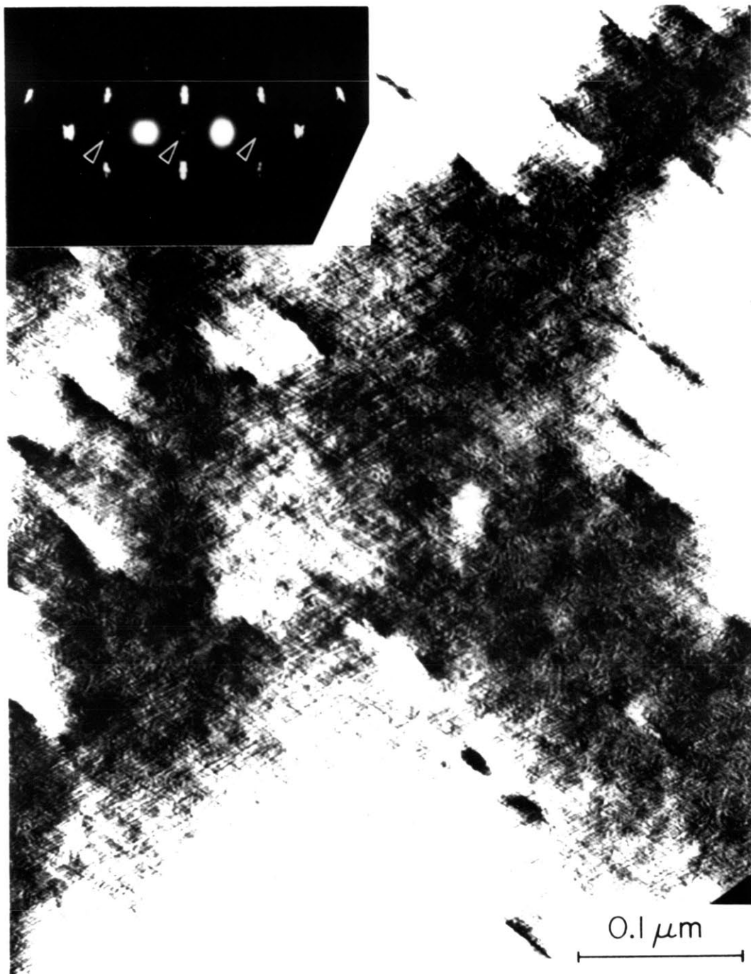
Figure D-1. Bright field ( g = 020 ) image of martensitic Fe-15Ni-1C aged 2.75 hrs at room temperature. The beam direction is near [100], but tilted slightly about [010]. In the inset diffraction pattern, spots denoted by arrows are due to epitaxial oxide.
