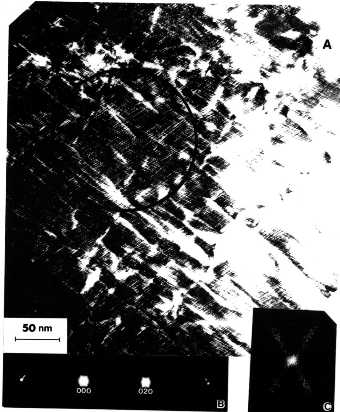
Figure 7-6. Martensitic Fe-15Ni-1C, aged 3 hrs at room temperature. (A) Dark-field transmission electron micrograph taken with the 020 reflection and its associated diffuse intensity. (B) Diffraction pattern. (C) Optical diffraction pattern from circled region in (A).
