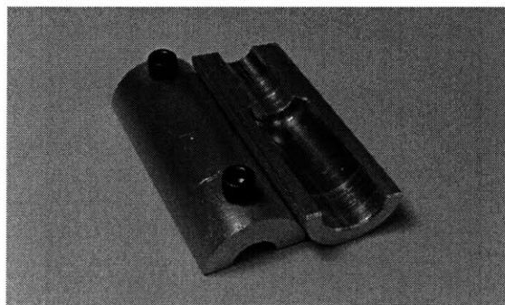
Figure III-15: Machined rigid alignment coupling for manufacturing assembly
